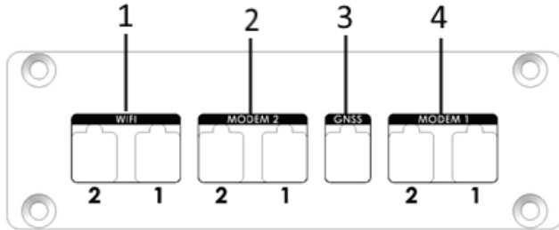
Figure 3 Rear Side of the WiCAR® (Configuration with 2 Modems, WLAN MIMO)
